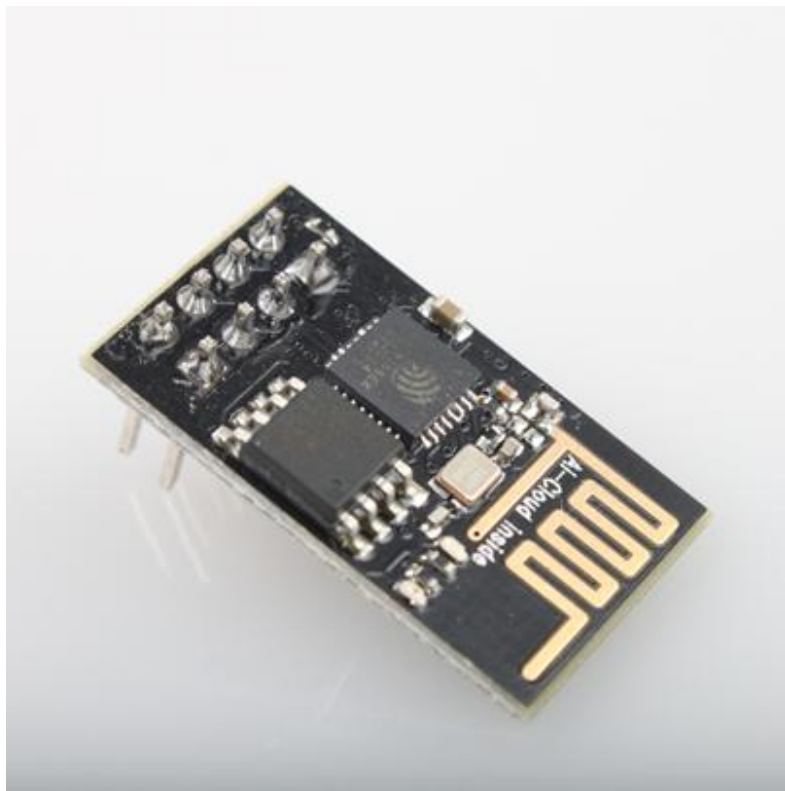
Figure 3 [Module Pin Counts, 8 pin, 14.3 mm *24.8 mm *3.0 mm]
